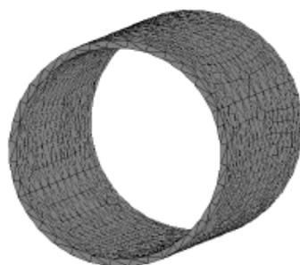
Figure 1. The domain of integration for the simulation of alginate reticulation in the real artery (*in-silico* model).
